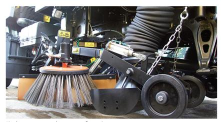
Single sweep or Dual sweep configuration. Trailed widesweep brush is adjustment-free and designed
