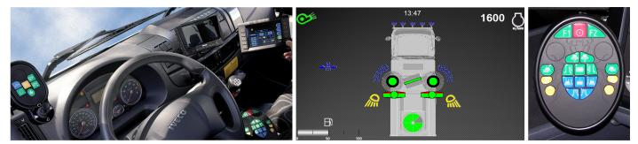
Scarab's CANbus control system has revolutionised the way sweepers are operated and maintained. Intuitive controls and a conveniently positioned colour monitor provide comprehensive levels of feedback to both operating and service personnel. A graphical display indicates the sweeping configuration and condition of the vehicle systems including warnings and regular service reminders. Real-time monitoring and data-logging provides valuable assistance in resolving problems and achieving
