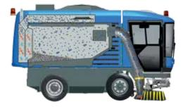
By doing this dust particles are electrically charged. This attracts them to the opposite charged collector and binds them together. These particles are then collected on the frame and are transformed into larger pieces of dust. These will then clog to the system until cleaned.
