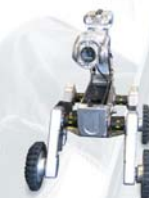
Mainline carriage accessory allows inspection of large-diameter pipes.
